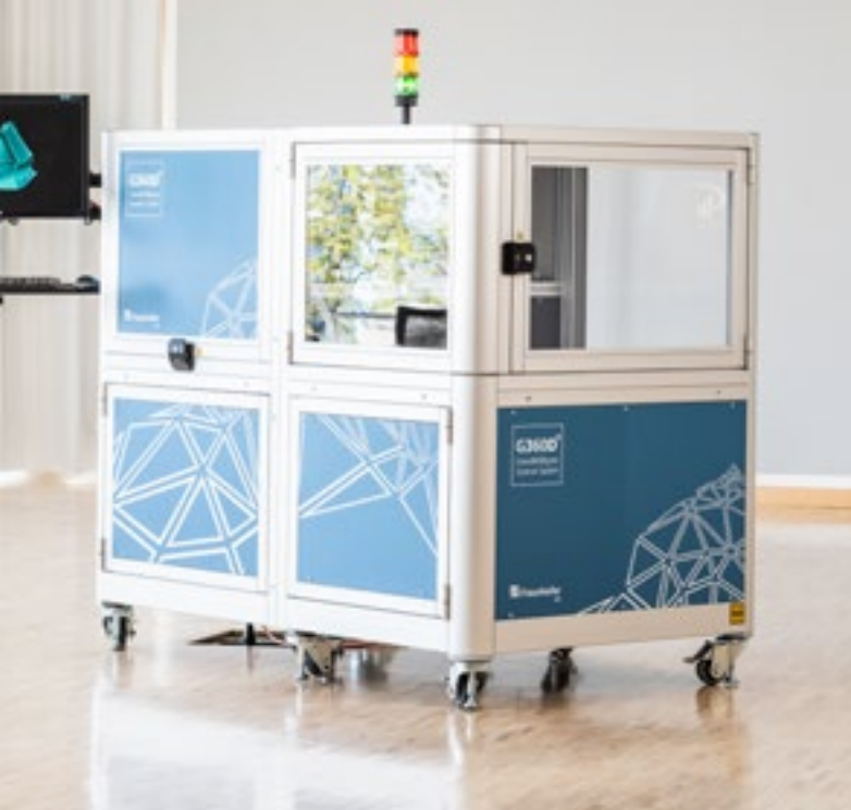
[3] goQUALITY3D-Demonstrator für Rundum-3D-Formvermessung. / goQUALITY3D demonstrator for all-round 3D shape measurement.
